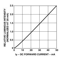
Figure 3. Relative luminous intensity vs. foward current.
