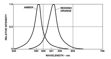
Figure 1. Relative intensity vs. wavelength.
