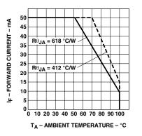
Figure 4. Maximum forward current vs. ambient temperature. Derating based on T Max = 110°C.
