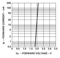
Figure 2. Forward current vs. forward voltage.
