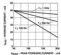
Figure 5. Maximum average current vs. peak foward current.
