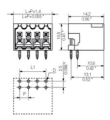
Order No. 1727930000 S2L 3.5/26/90G 3.5SN OR Part designation Version PCB plug-in connector, Male connectors, Soldered
