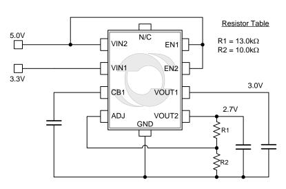
Figure 1 - Fixed / Adjustable Output Application
