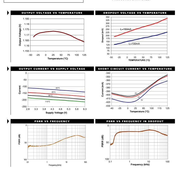
Typical performance characteristics, unless otherwise specified are:  $C_{IN} = C_{OUT} = 1 \mu F$ ,  $C_{BY} = 470 pF$ ,  $V_{IN} = V_{OUT} = 2.5 V$ ,  $T_A = 25 ^{\circ}C$ , ENABLE is tied to  $V_{IN} = V_{OUT} = 2.5 V$ ,  $V_{IN} = 2.5 V$ ,
