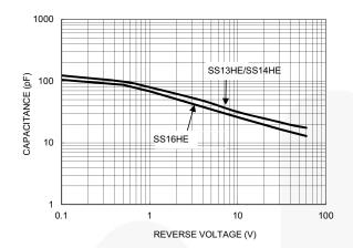
Figure 7. Typical Junction Capacitance
