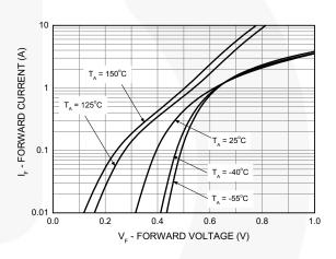
Figure 3. Typical Forward Characteristics - SS13HE / SS14HE
