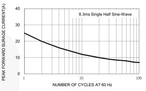
Figure 1. Forward Current Derating Curve
