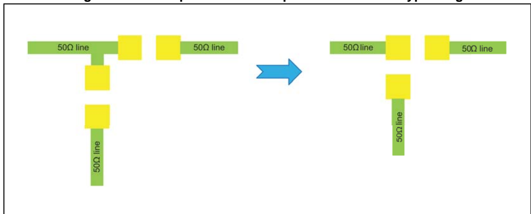
Figure 11. Reuse pads of one component on the line bypassing
