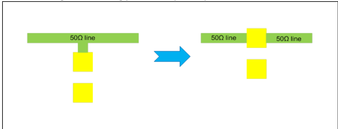
Figure 10. Placing parallel component pads on 50 ohms line
