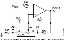
Figure 5. Noninverting Amplifier with Pseudologarithmic Gain
