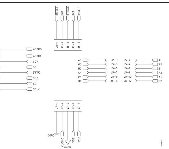
Figure 12. Schematic of Connectors to Daughter Board
