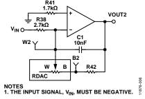
Figure 6. Inverting Amplifier with Linear Gain
