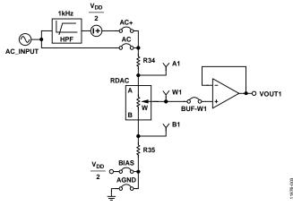
Figure 3. AC Signal Attenuator
