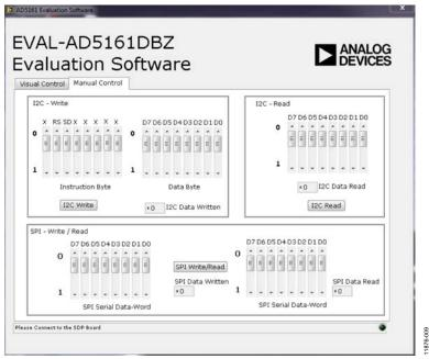
Figure 9. EVAL-AD5161DBZ Software Main Window, Manual Control Tab
