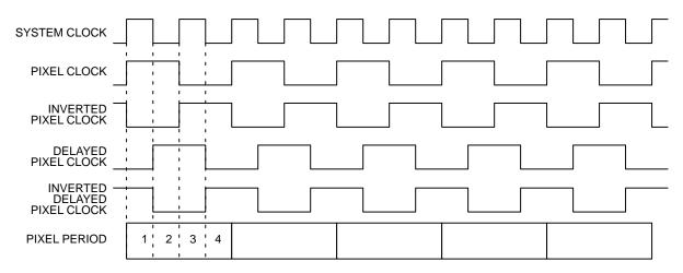
Figure 2. 30 MHz Pixel Clock Generation Timing
