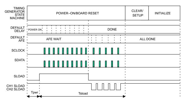
Figure 4. Power-On Initialization Timing
