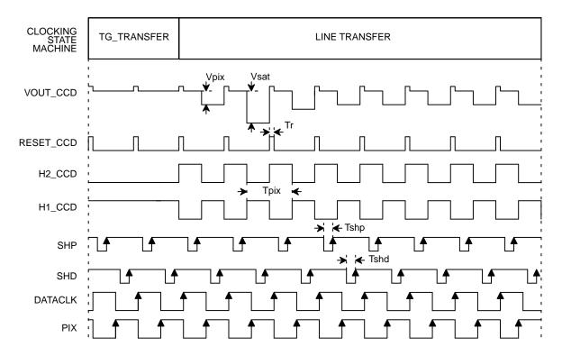
Figure 7. Horizontal Timing - Line Transfer
