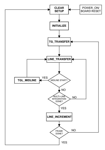
**Figure 3. Timing Generator State Machine**
