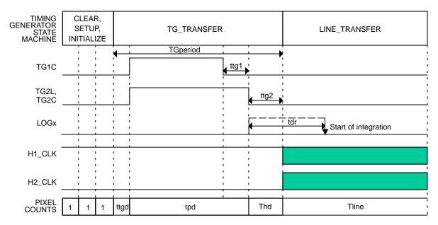
Figure 5. Transfer Gate Transfer Timing
