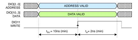
Figure 1. Programmable Register Timing
