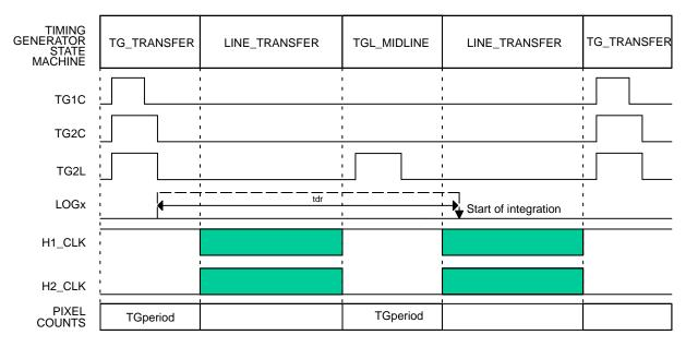
Figure 6. Line Timing – Single Line Integration Mode
