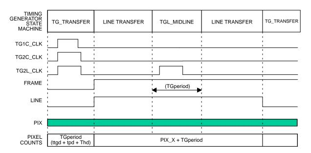
Figure 8. PCI-1424 Frame Grabber Timing - Single Line Integration Mode
