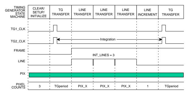
Figure 9. PCI-1424 Frame Grabber Timing - Multi-Line Integration Mode
