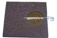
The longest leg of the LED should be placed on the side of the battery marked with the '+' sign. You can check this by gently holding the legs against the battery. If the LEDs lights then everything is the correct way around.
