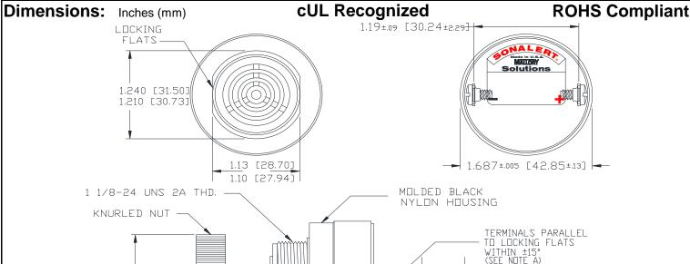
NOTE A: TERMINALS-.032 BRASS TIN PLATED, TAPPED FOR #6-32 SCREW. TWO #6-32 NICKEL PLATED BRASS SCREWS INCLUDED. WILL ACCEPT 1/4" QUICK CONNECT.
