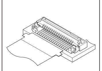
The connector for the 0.3mm thickness FPC with a mounting height of 1.3mm. FPC with protrusion prevents incomplete insertion and mis-insertion, so that it provides reliable connection.
