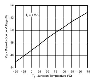
Drain Source Breakdown vs. Junction Temperature
