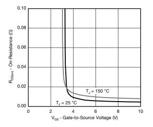
On-Resistance vs. Gate-to-Source Voltage
