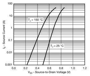
Source Drain Diode Forward Voltage
