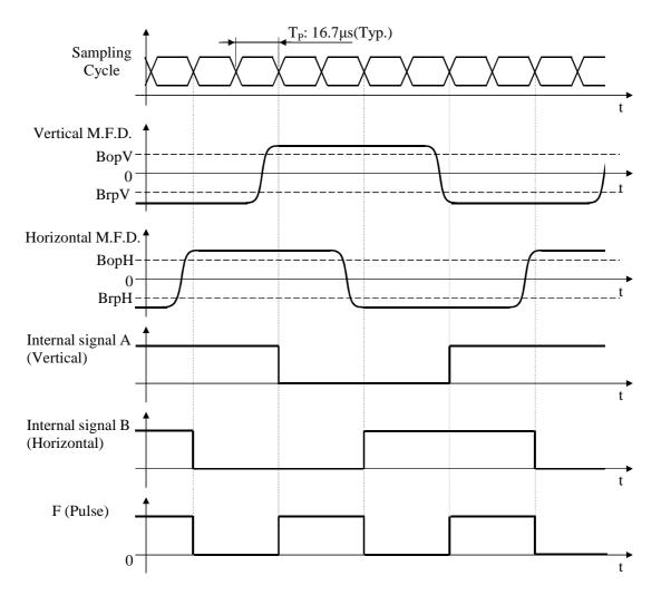
Figure 5. Timing diagram
