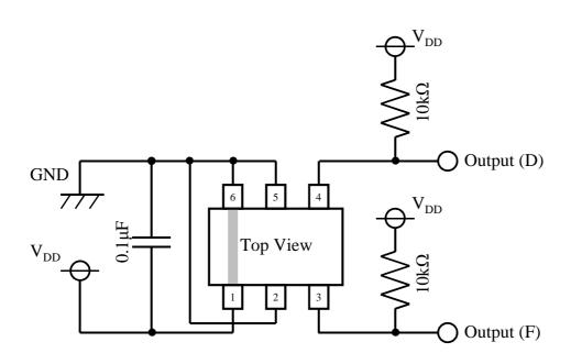
Figure 11. Recommended external circuit
