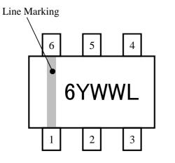
Marking is performed by laser Product name : 6 (AK8778B) Date code : YWWL Y : Manufactured year WW : Manufactured week L : Lot
