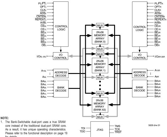
core instead of the traditional dual-port SRAM core. As a result, it has unique operating characteristics.
