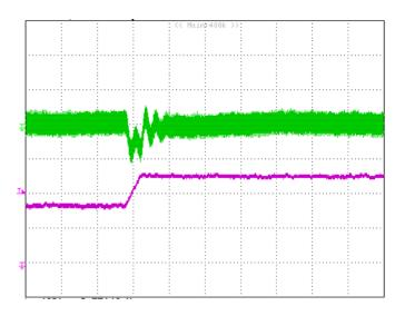
**Figure 9:** Output voltage response to step-change in load current (50%-75% of Io, max; di/dt =  $0.1A/\mu$ s, Vin=54V). Load cap: 10 $\mu$ F, tantalum capacitor and 1 $\mu$ F ceramic capacitor. Top Trace: Vout (200mV/div, 200us/div); Bottom Trace: Io (10A/div, 200us/div). Scope measurement should be made using a BNC cable (length shorter than 20 inches). Position the load between 51 mm to 76 mm (2 inches to 3 inches) from the module.
