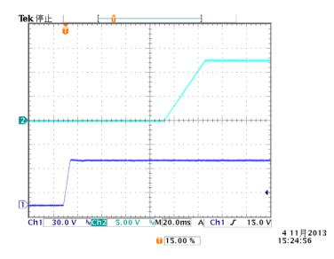
*Figure 6:* Turn-on transient at zero load current (10 ms/div), Vin=54V; Top Trace: Vout, 5V/div; Bottom Trace: input voltage, 30V/div;
