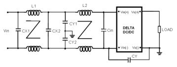
Cin is  $100uF^*2pcs$  low ESR Aluminum cap; CX1 is 2.2uF ceramic cap  $\times 2pcs$  in parallel;
