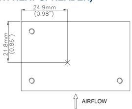
Figure 19: \* Hot spot temperature measured point. The allowed maximum hot spot temperature is defined at 105  ${\rm C}$
