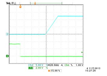
*Figure 4:* Turn-on transient at zero load current (10ms/div), Vin=54V; Top Trace: Vout, 5V/div; Bottom Trace: ON/OFF input, 2V/div;
