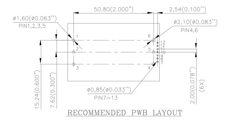
NOTES: DIMENSIONS ARE IN MILLIMETERS AND (INCHES) TOLERANCES: X.Xmm±0.5mm(X.XX in.±0.02 in.) X.XXmm±0.25mm(X.XXX in.±0.010 in.)
