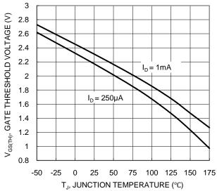
Figure 8. Gate Threshold Variation vs. Temperature
