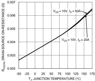
Figure 7. On-Resistance Variation with Temperature
