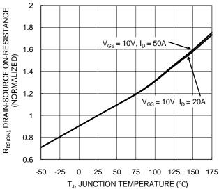
Figure 6. On-Resistance Variation with Temperature
