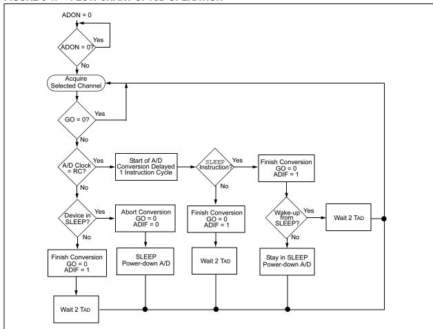
FIGURE 8-4: FLOW CHART OF A/D OPERATION
