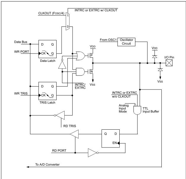
FIGURE 5-4: BLOCK DIAGRAM OF GP4/OSC2/AN3/CLKOUT PIN
