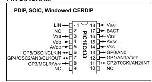
**Note:** Pins designated 'NC' have no internal connection to the device.
