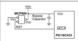
This brown-out protection circuit employs Microchip Technology's MCP809 microcontroller supervisor. The MCP8XX and MCP1XX families of supervisors provide push-pull and open collector outputs, with both high and low active RESET pins. There are 7 different trip point selections to accommodate 5V and 3V systems.
