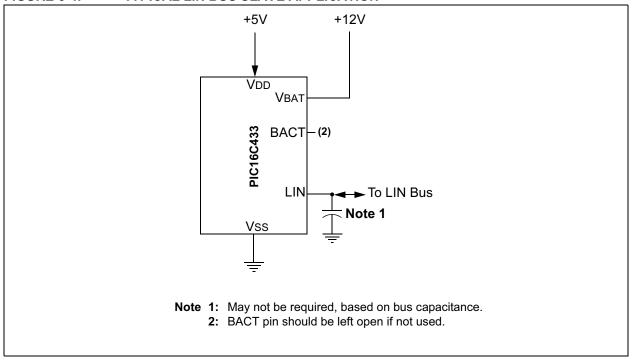
FIGURE 6-5: LIN BUS APPLICATION USING WAKE-UP INTERRUPT
