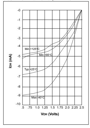
FIGURE 13-5: IOH vs. VOH, VDD = 3.5V
