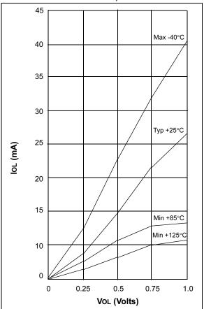
FIGURE 13-9: IOL vs. VOL, VDD = 5.5V
