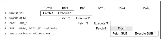
All instructions are single cycle, except for any program branches. These take two cycles since the fetched instruction is "flushed" from the pipeline while the new instruction is being fetched and then executed.
