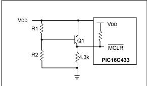
Note 1: This brown-out circuit is less expensive, albeit less accurate. Transistor Q1 turns off when VDD is below a certain level, such that:
