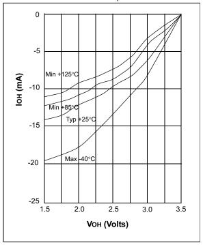
**FIGURE 13-6:** IOH vs. VOH, VDD = 5.5V
