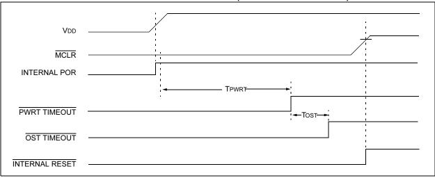
FIGURE 9-9: TIMEOUT SEQUENCE ON POWER-UP (MCLR TIED TO VDD)
