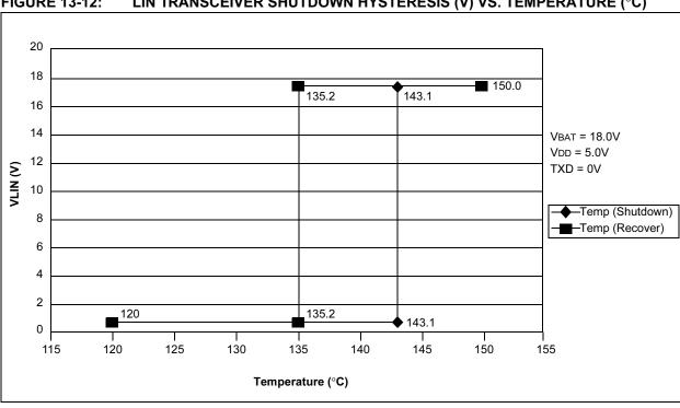
FIGURE 13-12: LIN TRANSCEIVER SHUTDOWN HYSTERESIS (V) VS. TEMPERATURE (°C)
