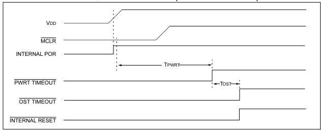
FIGURE 9-8: TIMEOUT SEQUENCE ON POWER-UP (MCLR NOT TIED TO VDD): CASE 2
