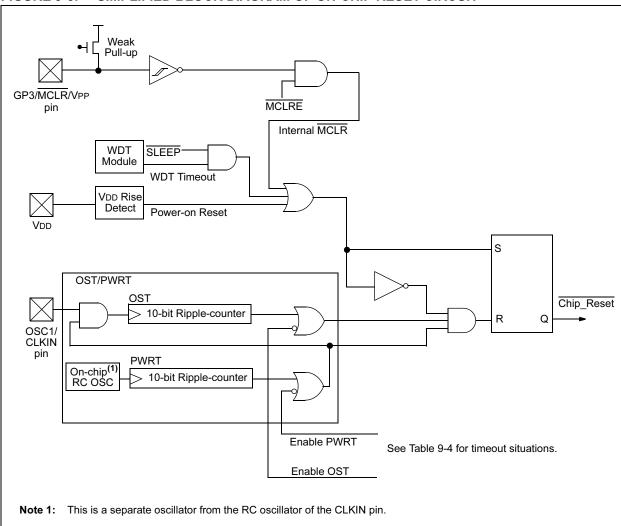
FIGURE 9-6: SIMPLIFIED BLOCK DIAGRAM OF ON-CHIP RESET CIRCUIT
