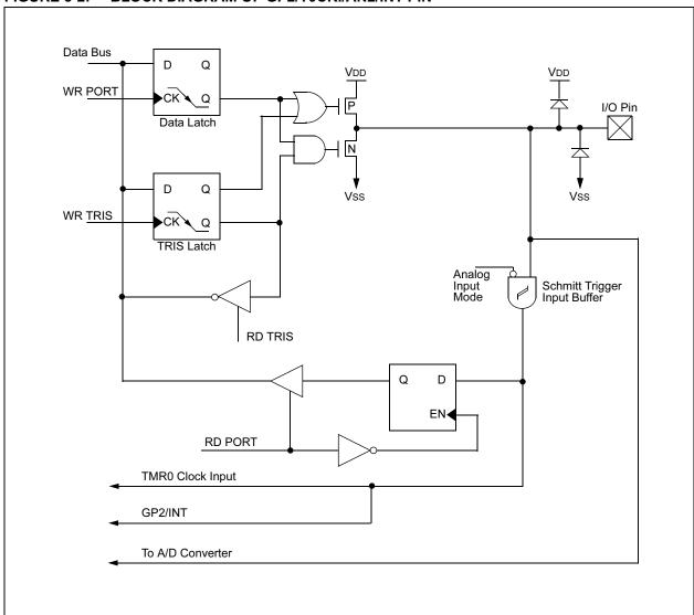
FIGURE 5-2: BLOCK DIAGRAM OF GP2/T0CKI/AN2/INT PIN
