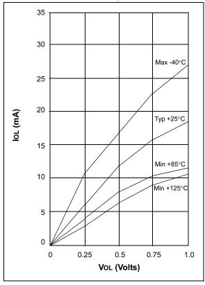
FIGURE 13-8: IOL vs. VOL, VDD = 3.5V
