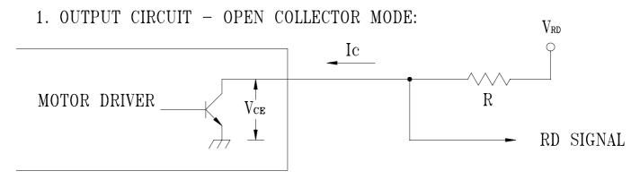
CAUTION: THE RD SIGNAL LEAD WIRE MUST BE KEPT AWAY FROM "+" LEAD WIRE & "-" LEAD WIRE.
