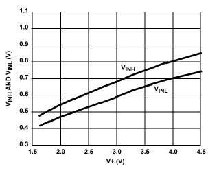
FIGURE 18. DIGITAL SWITCHING POINT vs SUPPLY VOLTAGE
