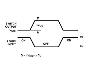
FIGURE 2A. MEASUREMENT POINTS
