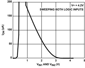
FIGURE 16. SUPPLY CURRENT vs VLOGIC VOLTAGE
